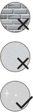
HUBBA PEBBLE mirrors must be mounted on dry, smooth, flat surface. Not for use on textured surfaces such as quartz & stone.
